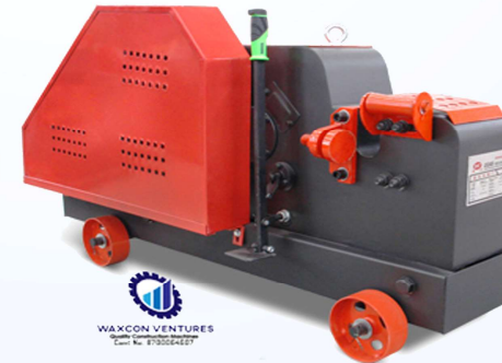
BAR CUTTING MACHINE MODEL: GQ50A, 52H CAP.: 8-42 MM POWER: 6.5 HP/ 4 KW WEIGHT: 525 KG
