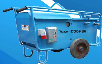
VACUUM PUMP Model WAXCON-50 Length 1200 mm Width 500 mm Height 800 mm Weight 110 Kg Max. Dewatering Capacity 24 sq. Mt within 30 min. Prime Mover Electric Power Rating 7.5 H.P Motor With Panel Board
