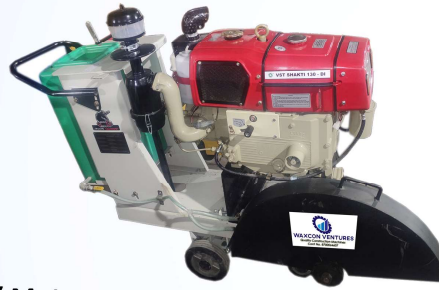
Concrete Cutter with Diesel Engine Power: 12.5 HP Cutting Cap.: 12 inch Depth Auto Water Running on Blade Blad Max. Dia: 750 mm
