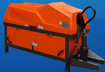
Steel Bar Straightner and Cutter Machine Straight capacity: 5-14mm Cutting Error: ±5mm Motor Power: 7.5 kw-3 Phase Dimention: 1840x610x1050 mm Pulling Speed: 24-60 m/Min Noise Value: <80db Weight: 245kg
